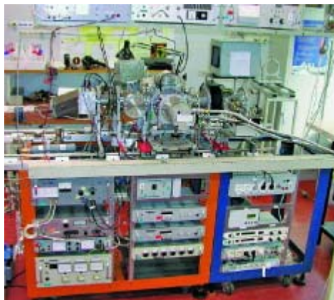
TOUR DE FORCE The LIR setup used to obtain \text{CH}_5^+ 's IR spectrum is a bench including an ultra-high-vacuum chamber and ion source (left), a 22-pole ion trap mounted on a helium refrigerator (center), and an ion-counting detector (right). The setup is axially transparent, so laser light from the FELIX free-electron laser can reach the trap after being introduced on the right side.
