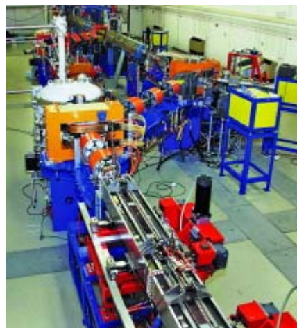
RAD SOURCE This free-electron laser at the FELIX Facility ( www.rijnh.nl/felix ) was used to generate IR radiation for experiments on \text{CH}_5^+ .
